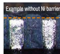
Example without Ni barrier Solder rises horizontal area
