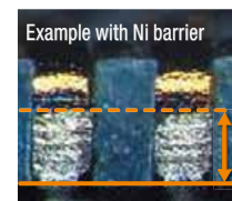
Example with Ni barrier Ni exposure part Limit of solder rise.
