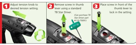
The EVO 9 quick-adjust tension feature allows for easy, blind tension adjustments; useful when using more than one cable tie type during an assembly application.
